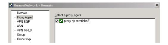
When the check box is selected, it confirms the Network Processor assignment as a Proxy Agent for that domain.
