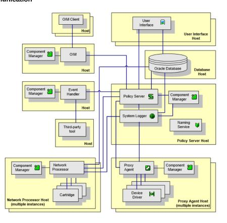
Figure 9-1 Standard Configuration of Component Distribution and Communication
