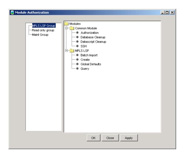
After selecting access to the Batch Import, Create and Query functions for the group (but not the Global Defaults function), the GUI looks like this:
