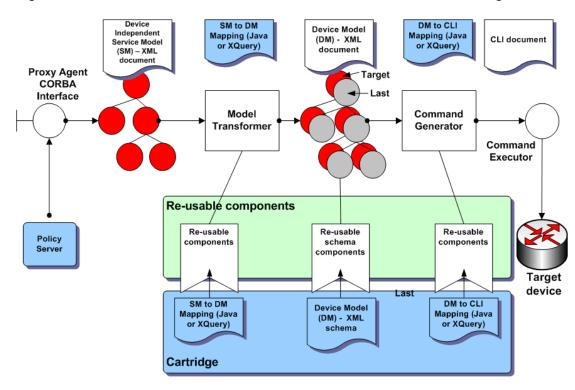
Figure 7-3 Network Processor Data Flowchart from the Interface to the Target Device
