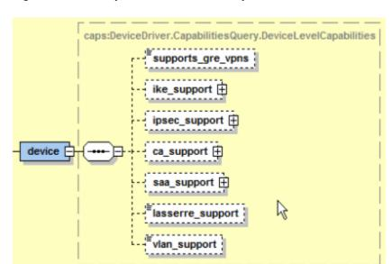
Figure 7-5 Example of Device Level Capabilities
