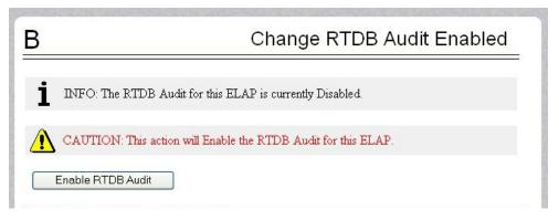
If the Information field indicates that the RTDBLSMS HS Audit for this ELAP is currently Disabled (as shown in Figure B-2), click the Enable RTDBLSMS HS Audit button.
