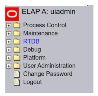
If the ELAP that you logged into is not Active, and the other ELAP is active, select **Select Mate** from the main menu. (If both ELAPs are Standby, correct the situation preventing one ELAP from taking the active role, and repeat this step.)
