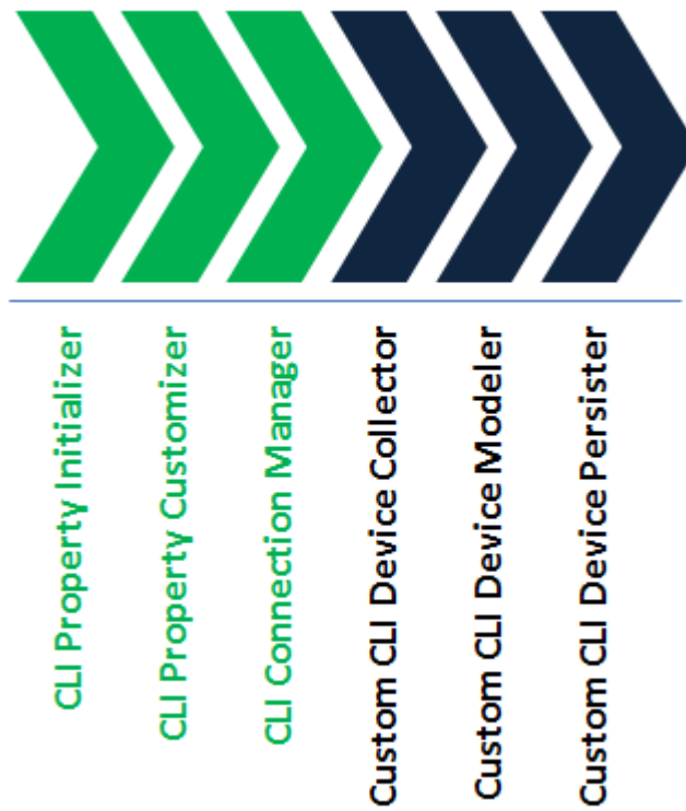
Figure 2-3 New Custom Processors Workflow
