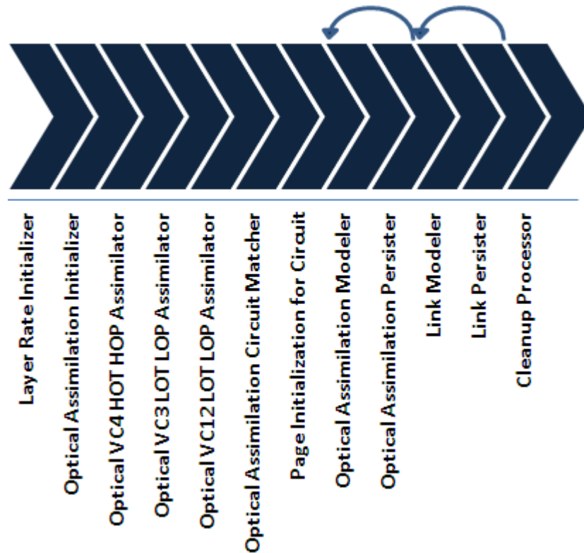
Figure 2-1 Assimilate Optical Circuits Processor Workflow
