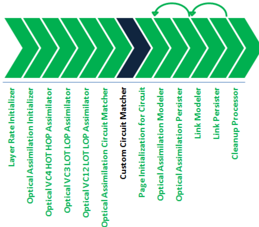
Figure 7-1 Custom Circuit Matcher Processor Workflow
