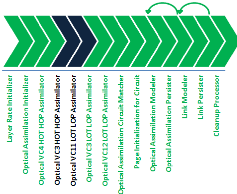
Figure 7-2 SONET Assimilation Processor Workflow
