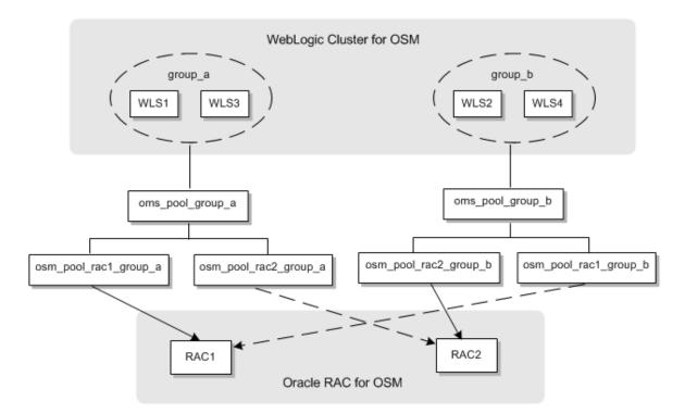
Figure 8-4 Data Source Configuration for Oracle RAC Active-Active
