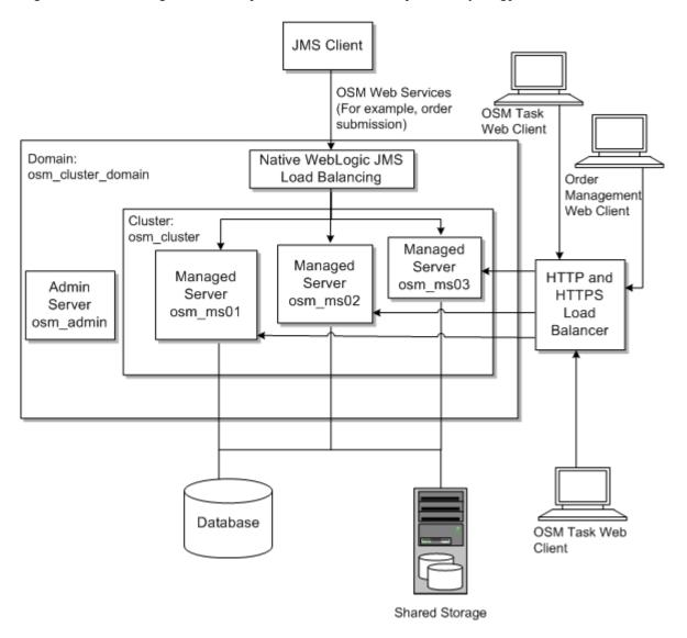
The system includes a WebLogic Server cluster with four managed servers, an administration server, a JMS client sending orders to OSM, and an HTTP load balancer that load balances HTTP and HTTPS messages to OSM from various
