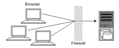
In this topology, all the application components and data are kept on a single server, protected from external attacks by a firewall. The firewall can be configured to block known illegal traffic types. There are fewer resources to secure because all the components are on a single server and all of the communication is local. Fewer ports have to be opened through the firewall.
