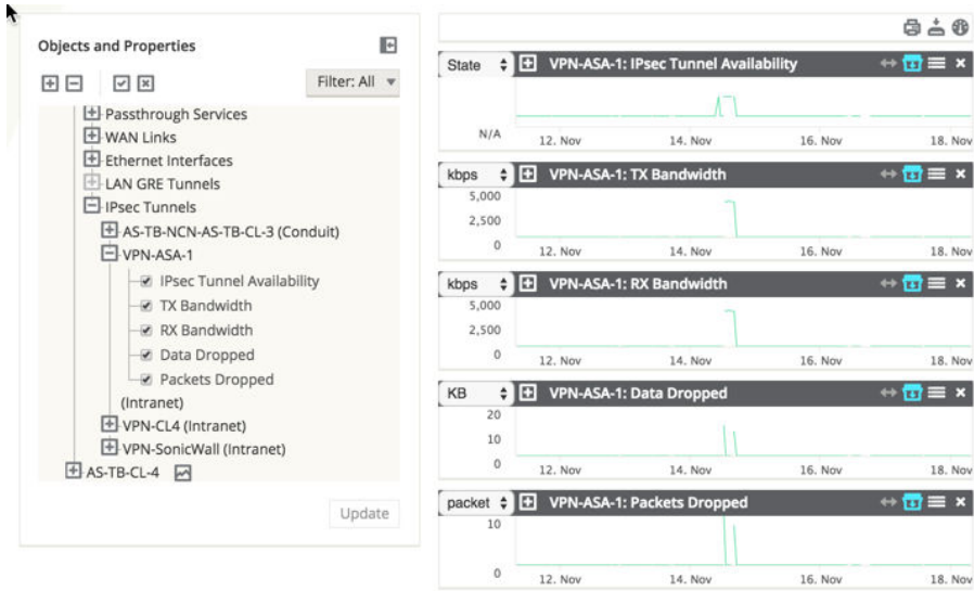
Figure 6: IPsec Tunnel Graphs
