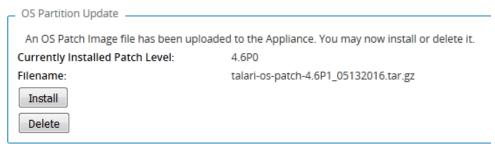
7. Wait for installation to complete. You will then be returned automatically to Manage Appliance → OS Partitions, where the patch version (e.g., 4.6P1) will now be displayed as the active version in the OS Partition Versions section.
