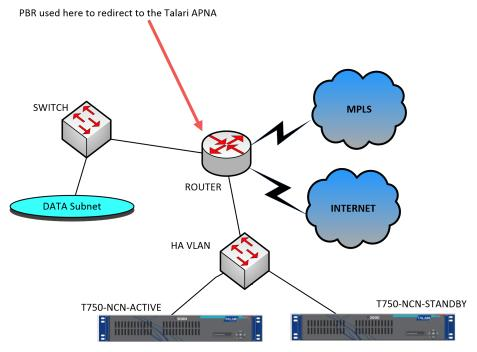
In One Arm mode it is recommended that the Talari Appliances do not reside in the data network subnets. This means the Talari Conduit traffic doesn't have to traverse the PBR and avoids route loops,
