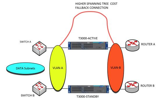
routable VLANS are recommended to ensure the LAN side switches and WAN side routers are reachable at Layer 2.
