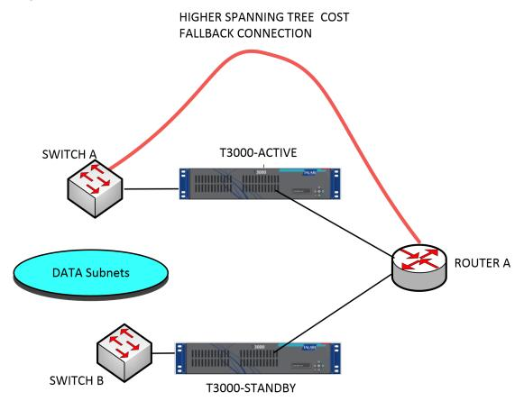
In the above diagram, only one path through the Active appliance is used. It is important to note the bypass interface groups are configured to be fail-to-block and not fail-to-wire so that we don't get spanning tree loops during a failover.
