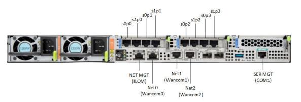
Figure 2-13 Oracle X8-2 Configuration B (One QSFP and One 4x10 GigE NICs)
