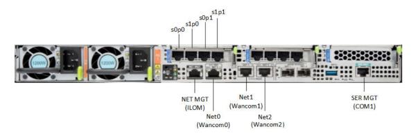
Figure 2-12 Oracle X8-2 Configuration B (Two 4x10 GigE NICs)
