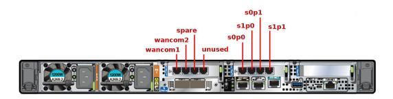
Figure 3-2 Oracle Server X9-2 Configuration B: four-port 10-Gigabit QSFP+ NIC
