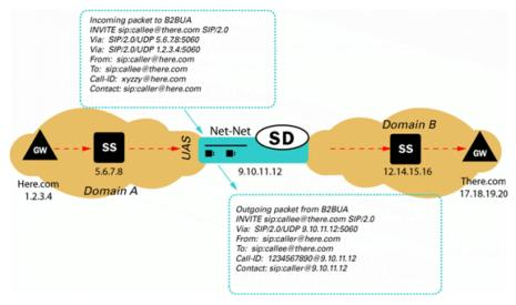
Access - In an access model the SBC is contacted by a SIP endpoint to relay endpoint signaling information. The IP address of the endpoint is usually not known, so trust should be established through behavior such as establishment of a successful registration. Once the endpoint becomes trusted, dynamic Access Control Lists (ACL) and Call Admission Controls (CAC) can be applied. Monitoring of potentially abusive behaviors provides a mechanism to "demote" or place endpoints on a blocklist.
