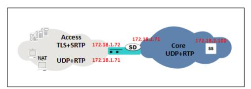
Secured-network parameter is set to ENABLED under the access sip-interface and ENABLED on the core sip-interface. Only one security-policy is configured for SRTP under 172.181.72. Two media-sec-policies are created, one in the access network with mode=any and one in the core with mode=RTP. As in the access network both RTP and SRTP endpoints could be present, the egress-offer-format is set to simultaneous-best-effort.
