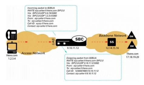
Hybrid - A hybrid model combines both Peering and Access topologies into a single configuration. This is a fairly common model, where remote users use a registrar server in the core network, but their calls are forwarded to a service provider on one of the peer connections.
