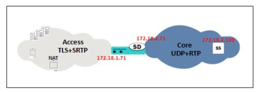
The IP used for SIP and SRTP in the SBC in the access network is 172.18.1.71, and the IP used for SIP and RTP in the core network is 172.18.2.71. The SIP Registrar/Proxy in the core network is in 172.18.2.100.
