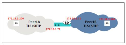
In the SBC, 172.18.1.71 will be used for SIP (TLS) and SRTP in the peer1A network, while 172.18.2.71 will be used in the 172.18.2.71.
