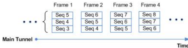
Figure 21-16 Redundancy — DTLS/UDP Redundancy
