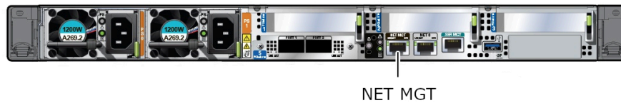
Figure 5-14 Connecting to ILOM over the Network
