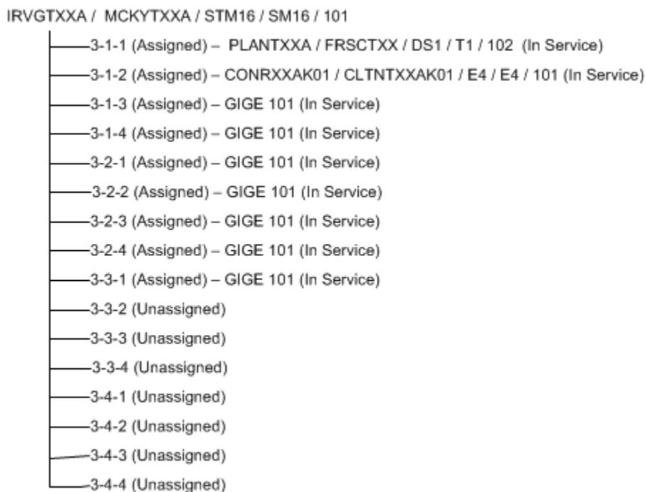
Figure 14-25 Intra-Facility Grooming: After
