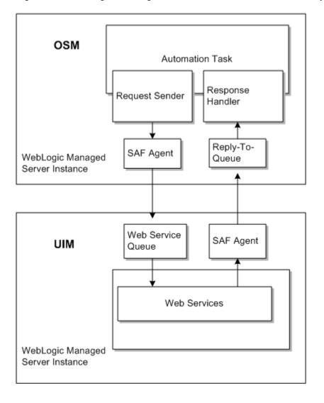
Figure 6-1 SAF Agent Configuration Between UIM and a Remote Application (OSM)
