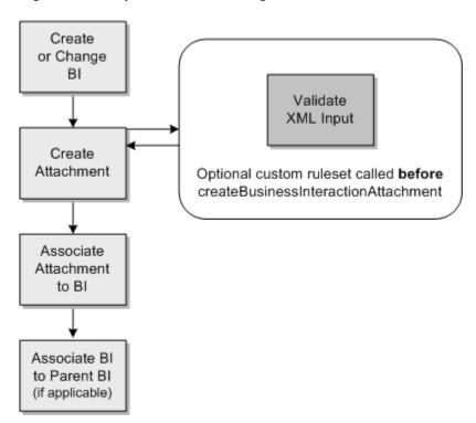
Figure 2-2 CaptureInteraction Logic Flow
