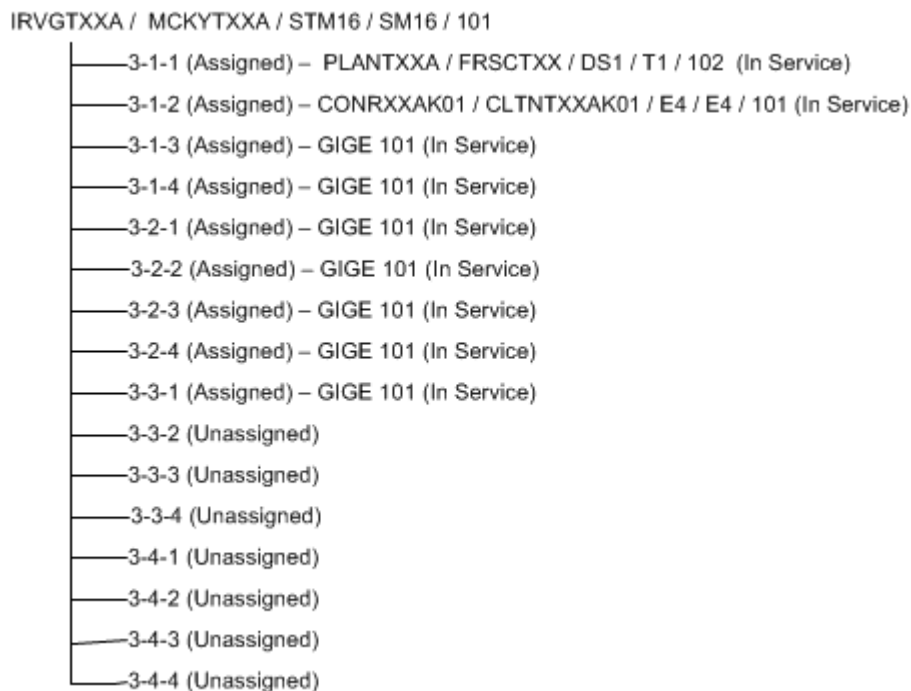
Figure 14-25 Intra-Facility Grooming: After
