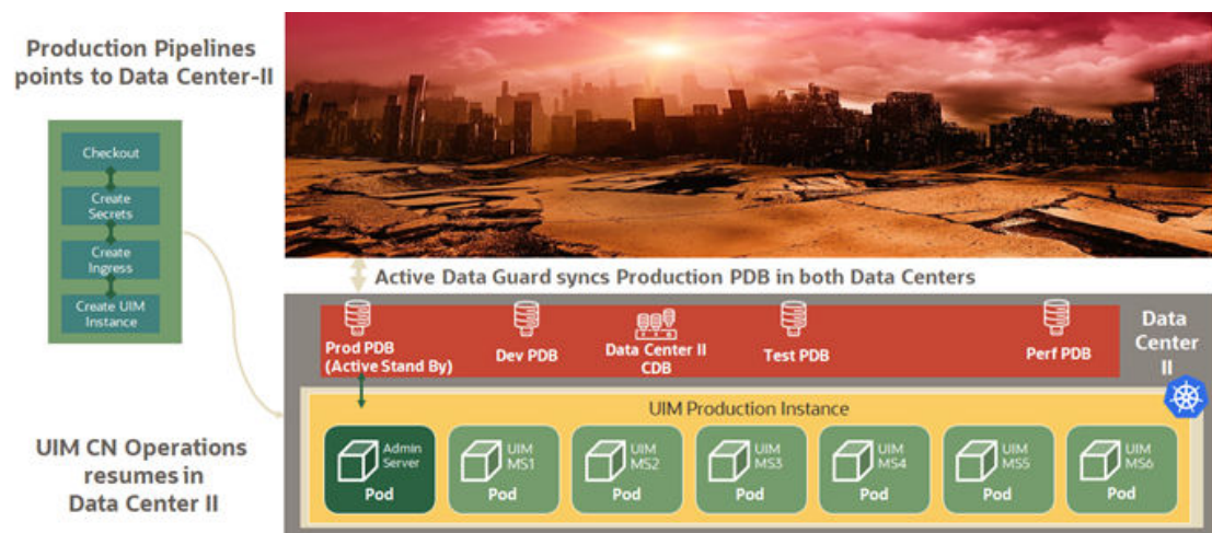
Figure 14-6 Active-Passive Deployment During Disaster and Recovery
