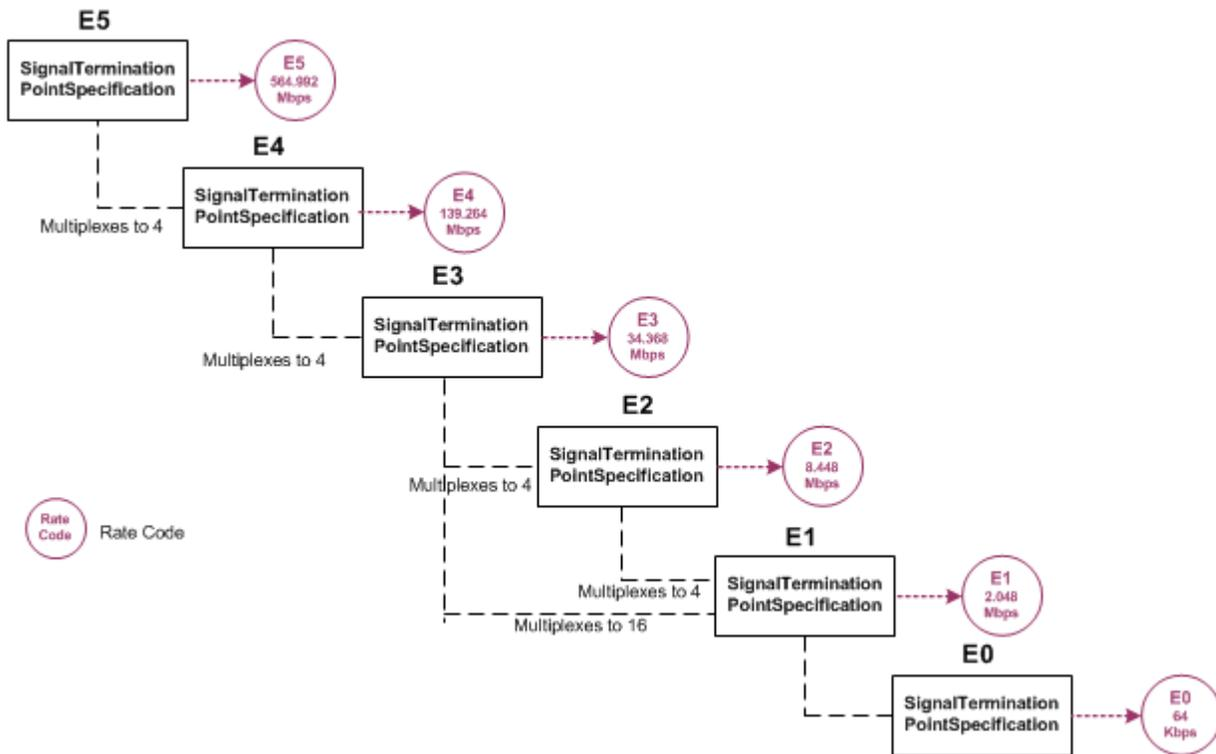
When you associate a rate code to a Connectivity entity, you determine the signal that applies to the facility represented by the entity and also determine its multiplexing options. For example, if you create a Connectivity entity with the E4 rate code, the facility can be multiplexed only to E3 channels.
