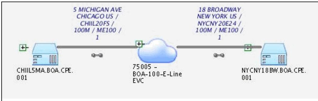
The service connectivity is enabled by UNI connectivities on the service location ends and network transport inside the service provider networks. [Figure 16-8](#) illustrates the design of the service connectivity shown in the previous figures.
