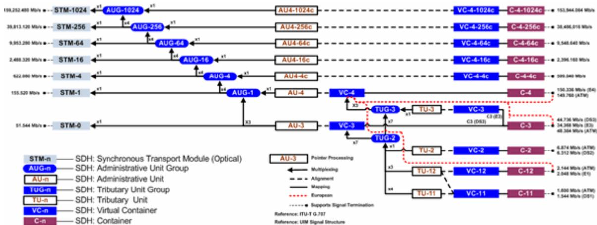
When you set up a hierarchy of device interfaces to support an SDH facility, however, you need to include only the interfaces on which channels are actually terminated. These interfaces include VC4, VC3, VC12, and so on. These are the interfaces that are interconnected to other interfaces when an enabling connectivity is passed through a logical device. Figure 14-7 illustrates the channel and device interface hierarchy for an STM1 facility.
