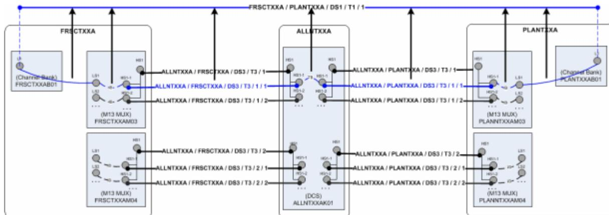
Figure 14-27 illustrates the situation after grooming has taken place. FRSTXXXA / PLANTXXXA / DS1 / T1 / 1 is now enabled by channels on other multiplexers at the same network locations and by interface-bound cross-connects between interfaces. UIM has automatically created a trail-bound interface between interfaces on the ALLNTXXXK01 DCS. (The trail-bound cross-connect used to enable the trail previously has been removed.)
