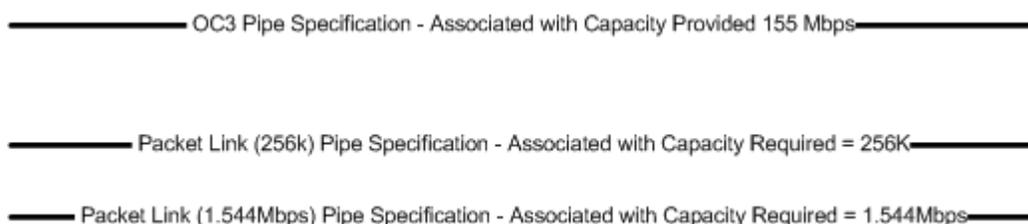
For example, you can define an OC3 Pipe using the Capacity Provided entity that provides bandwidth of 155.52 Mbps, 100% of which can be consumed. Pipes that can use that capacity are associated with capacity-required entities.
