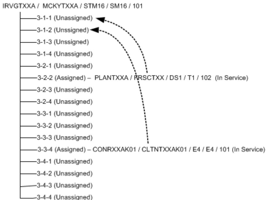
With these changes, a large contiguous block of channels becomes available, making it possible to assign them to the Ethernet pipe. [Figure 14-25](#) illustrates these assignments.
