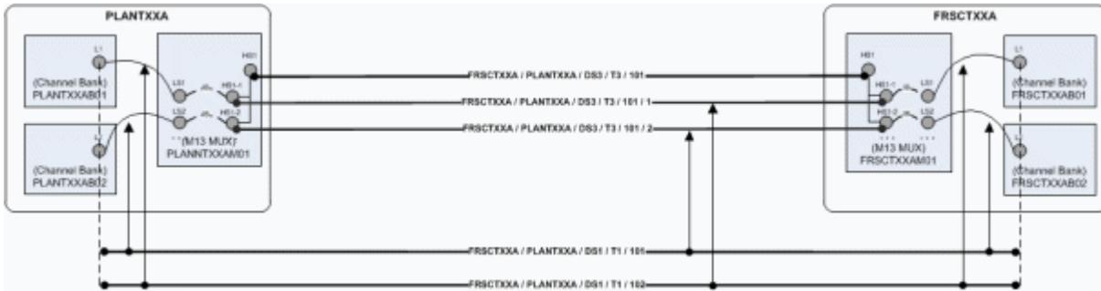
A new device and location are inserted between the PLANTXXA and FRSTXXA locations, resulting in the creation of two new T3 facilities to replace the previous T3.
