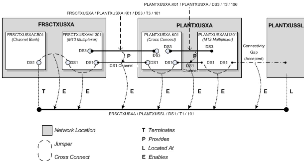
In this example, the FRSTXUSXA / PLANTXUSSL / DS1 / T1 / 101 facility is terminated on a device interface in a channel bank located at the network location FRSTXUSXA. Seven segments are required to complete the end-to-end connectivity path:
