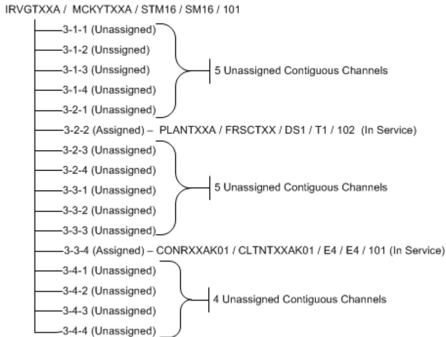
To free the required number of contiguous channels, the STM16 facility must be groomed. The channel assignments of the two E4 connectivities must be moved to make 7 contiguous channels available. The required changes are illustrated in [Figure 14-24](#).
