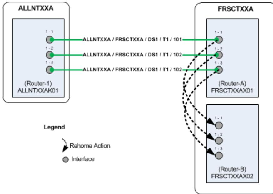
Rehoming a facility requires changes to the termination of the facility itself and to any channels it provides. Channels are re-terminated on sub-device interfaces provided by the new device interface on which the facility is terminated.
