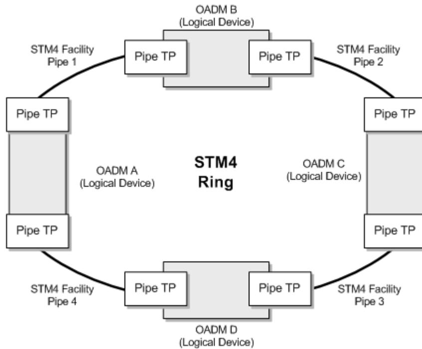
To enable an E1 service trail from OADM A to OADM C with both a primary path and a secondary path, you can use two connectivity paths:
