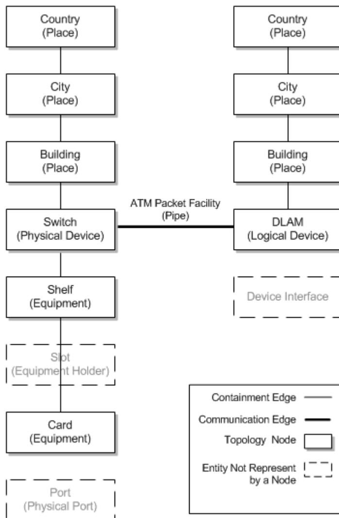
Connectivity is shown first at the level of the places to which connected entities are associated. In this case, that is at the level of the Place entities that represent the buildings in which the switch and DSLAM are housed. If the switch and DSLAM had been associated with the City locations, connectivity would be shown at that level.
