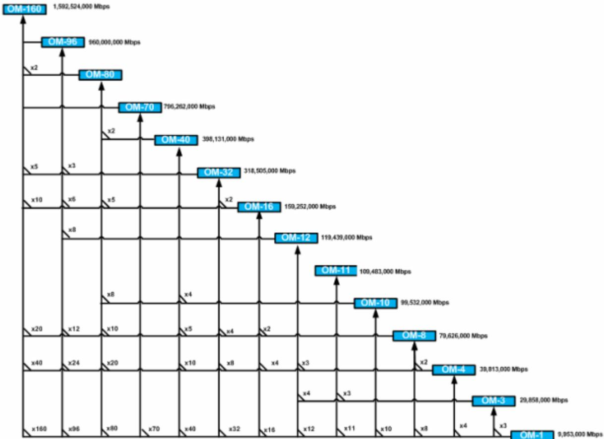
You can use WDM channels to enable other connectivities. For example, you can enable an OC192 SONET facility with an OM1 (10 Gbps) channel or a 100 Gbps Ethernet pipe with an OM10 channel.
