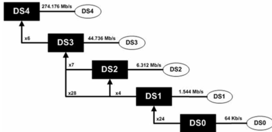
Figure 14-4 illustrates the hierarchy of channels that a connectivity requires to represent a T1 facility. The DS1 device interfaces on which the facility is terminated must include 24 DS0 sub-interfaces on which to terminate the channels.
