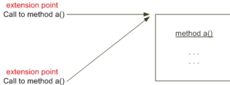
Figure 8-6 represents a ruleset configured to run after the method. For this type of configuration, the extension point is weaved into the UIM code stream, immediately after the method call. The result is the ruleset custom code runs after the method runs.
