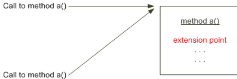
Figure 8-3 represents a ruleset configured to run after the method. For this type of configuration, the extension point is weaved into the method, immediately following the last line of the method's executable code. The result is the ruleset custom code runs after the method runs.
