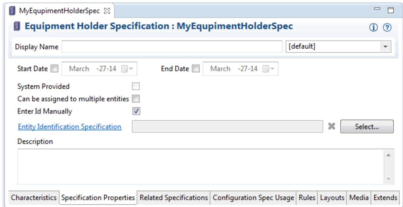
When the **Enter Id Manually** check box is deselected, it indicates that when creating an instance of the specification in UIM, the **id** attribute value is automatically generated. In Figure 2-9, the **Enter Id Manually** check box is deselected, and the option to select an Entity Identification Specification is now enabled.
