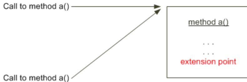
Figure 8-4 represents a ruleset configured to run instead of the method. For this type of configuration, the extension point is weaved into the method, and the method's executable code does not run. The result is the ruleset custom code runs instead of the method.
