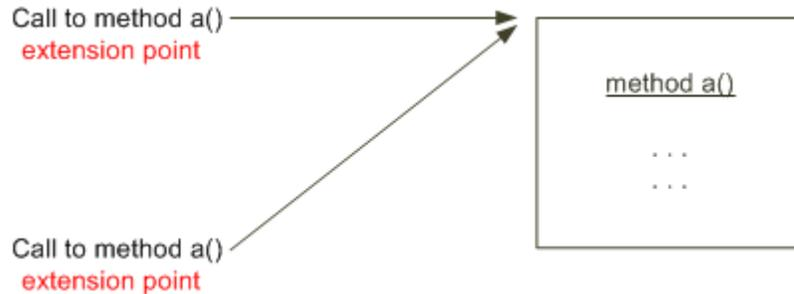
Figure 8-7 represents a ruleset configured to run instead of the method. For this type of configuration, the extension point is weaved into the UIM code stream, and the method is not called. The result is the ruleset custom code runs instead of the method.
