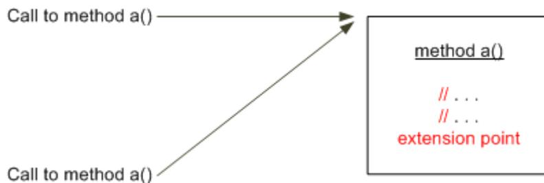
Figure 8-5, Figure 8-6, and Figure 8-7 show an extension point type of call, which dictates the extension point is weaved at the call to the method defined by the extension point. For this
