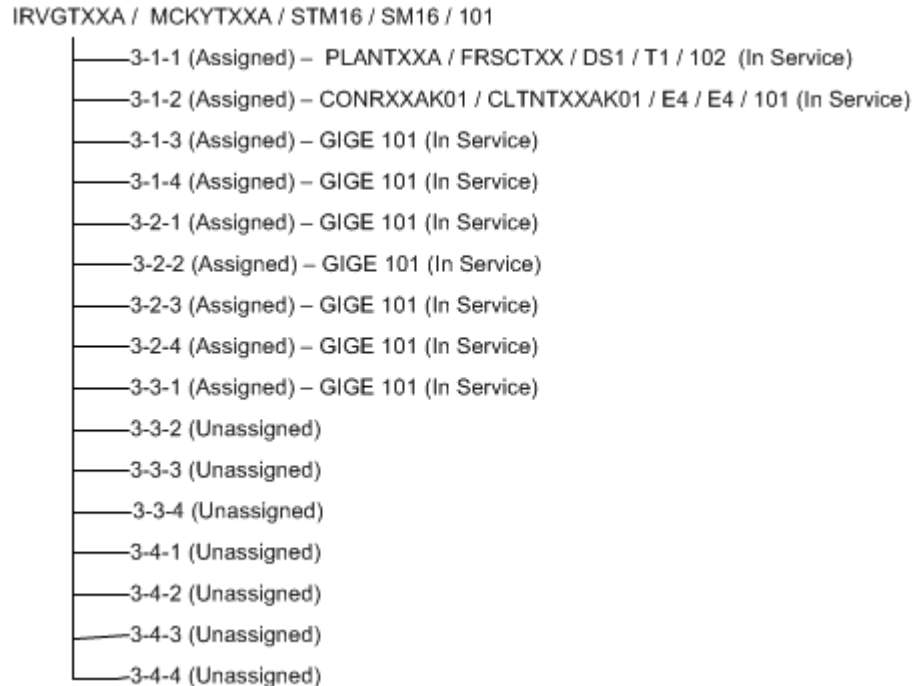
Figure 14-25 Intra-Facility Grooming: After
