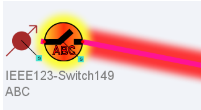
Example: Switch Warning and Conductor Violation
