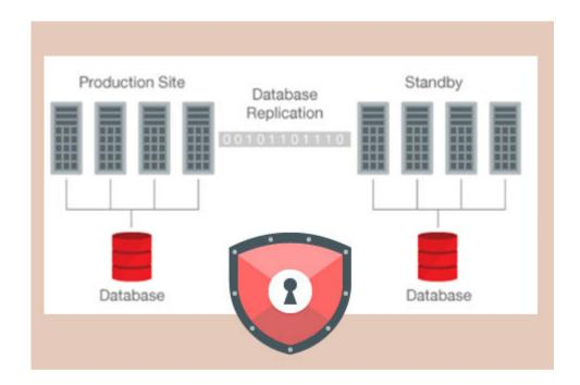
Under normal operating conditions, Active Data Guard replicates changes made in the primary database instance to the secondary database instance on a transactional basis (i.e. as changes are committed to the database).
