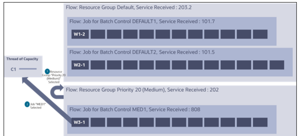
Figure 3-9: Three Jobs Competing for Backlogged Threads
