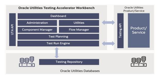
Oracle Utilities Testing Accelerator's workbench can be accessed using a web browser, such as Firefox or Google Chrome. The workbench allows to create and manage components and flows. Additionally, flow runs and their corresponding history can be managed from the workbench. There are various modules within the workbench:
