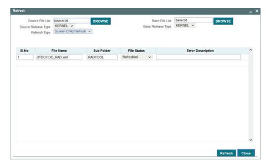
The figure above shows the content of the **source.txt** file. Here **UTDCIFDC** is the child RADXML that has to be refreshed. If a child refresh of more than one function id is required, the absolute path of each child RADXMLs has to be specified, each in a new line.
