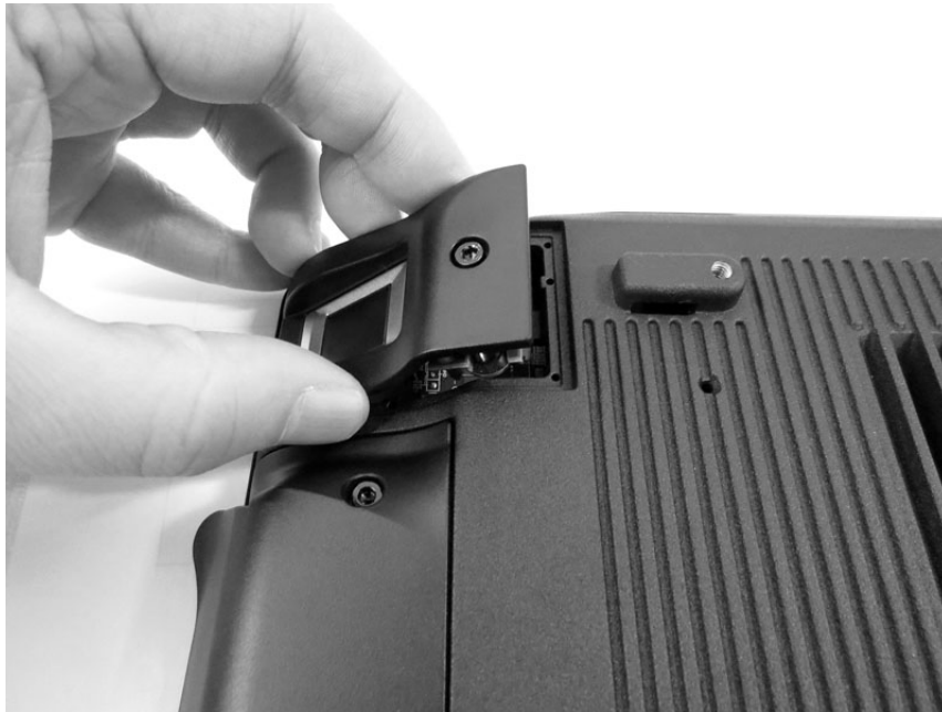
Figure 3-19 Installing the Fingerprint Module
