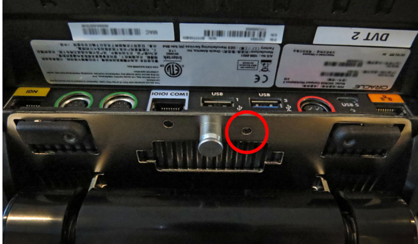
Figure 3-4 Location of the Compact Workstation 3 Series Security Screw
