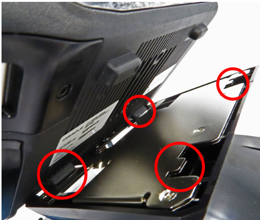
Figure 3-3 Mounting the Compact Workstation 3 Series on the Flexible Stand
