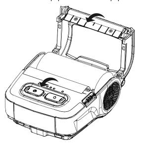
4. Tear off any excess paper toward the side of the printer.
