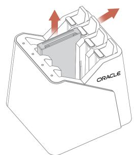
Press the battery release and remove the battery
