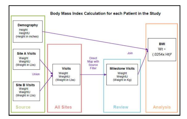
Figure 4-1 Transformation Example: BMI Calculation
