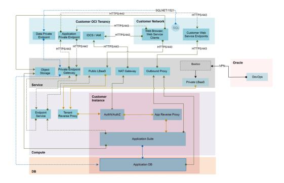
RAP services are deployed within a managed Kubernetes cluster, providing isolation for each customer instance. Each tier of the infrastructure is isolated by OCI Virtual Cloud Network (VCN) traffic ingress/egress lists.
