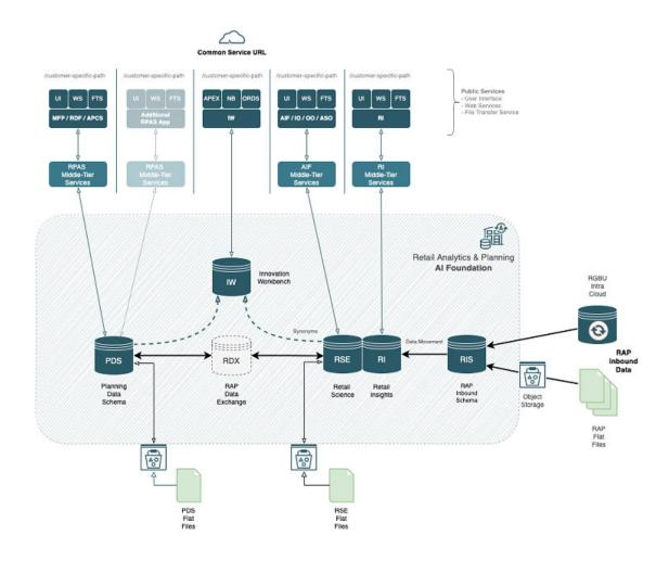
The above diagram shows the high-level RAP Architecture. The customer can upload their main input files as RAP Inbound Data using Object Storage and from their Planning
