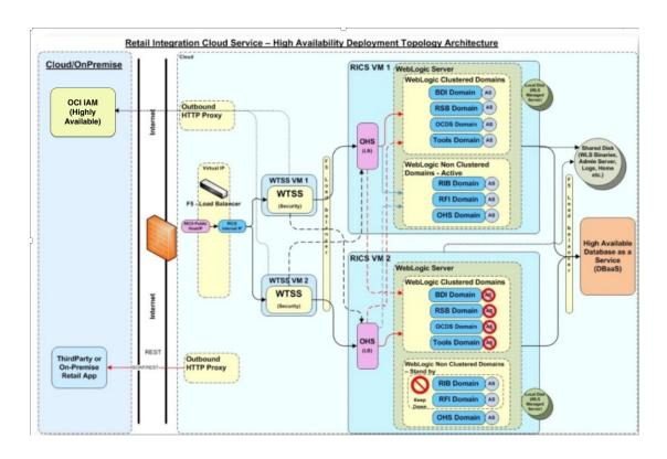
Most customer access to the Integration Cloud Service is via the web tier. The web tier contains the perimeter network services that protect the Integration applications from the internet at large.
