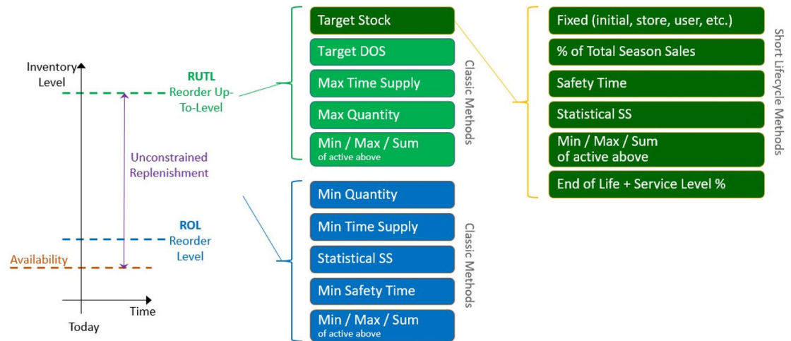
Figure 20-13 Point in Time Replenishment Methods
