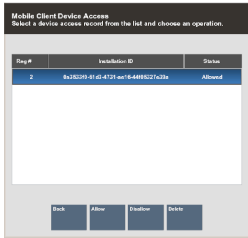
Figure 25-9 Mobile Client Device Access Screen
