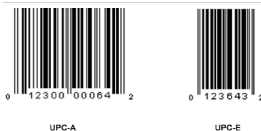
Figure E-1 UPC-A and UPC-E Differences
