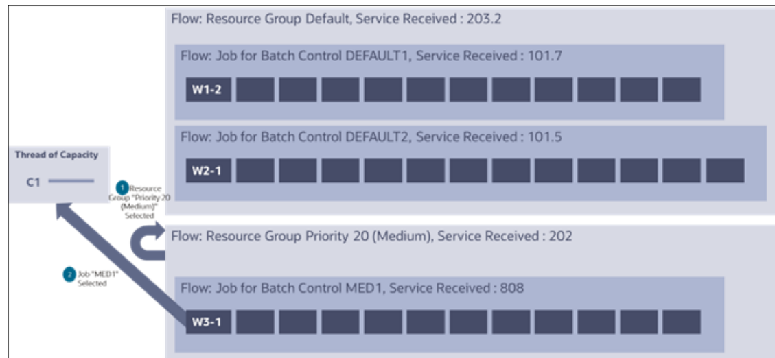
Figure 3-9 Three Jobs Competing for Backlogged Threads
