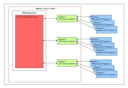
Both the OEM's OPC UA client-server application and the LEC Server instances have redundant servers at the Main Control Center, so if one instance fails, the system can fail over to the redundant application on another machine.
