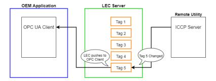
After reading the tagged value, the OPC UA client can be programmed to prevent or allow the issuing of a control directive (Block 5) to the remote ICCP server.
