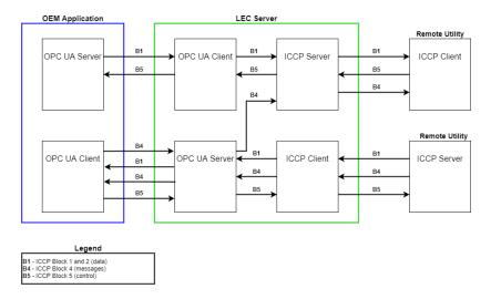
The top dataflow shows an application's OPC UA server communicating with a remote ICCP client using an LEC Server instance as the ICCP Front End (IFE). This communication transmits both Blocks 1 and 2 and Block 5 data. Blocks 1 and 2 transfer measurement and state information from a local ICCP server to a remote ICCP client. Block 5 provides for the transfer of control information from the remote ICCP client to the local ICCP server.
