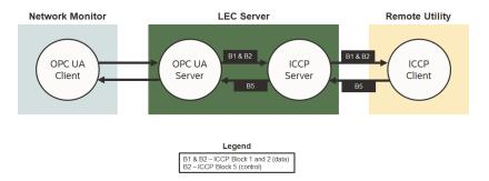
The conformance block data that the application's OPC UA client receives from the remote VCC server is outlined in <a href="this image">this image</a>. This data is received by the LEC VCC client, and then processed in the LEC Processor so that it is compatible with the OPC UA data types.
