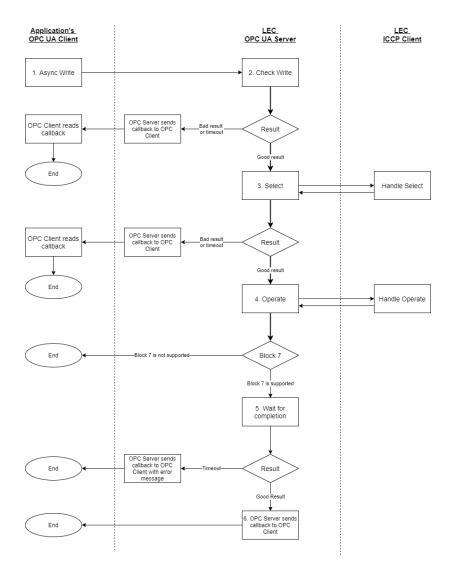
The following are steps required to issue a command or set a setpoint using the Select Before Operate protocol with and without Block 7 support.
