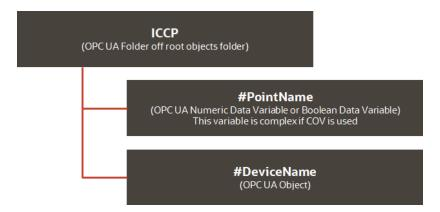
While ICCP is the default name for the root of ICCP data, this OPC UA folder name is the name of the configuration database file. Although only point values and change-of-value (COV) variables are shown above, you can configure variables for individual ICCP Quality tags by modifying the default batch file.
