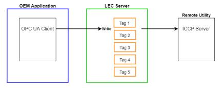
**Note**: Prior to working with tags, you need to understand it is always the remote ICCP server's view of the tag that is the actual tag state. Even if the OPC client writes to a tag, and it is sent to the ICCP server, the ICCP server can ignore the set tag and consequently will return its view of the tag state in the next get request.
