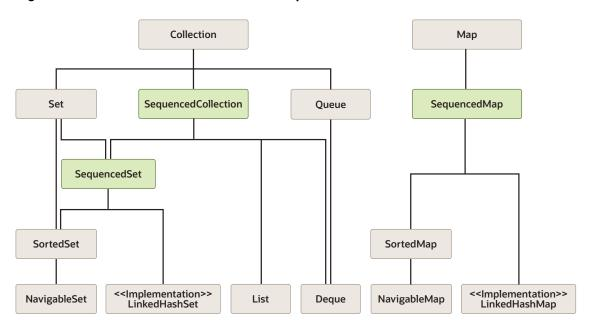
Figure 5-1 Collections Framework with Sequenced Interfaces
