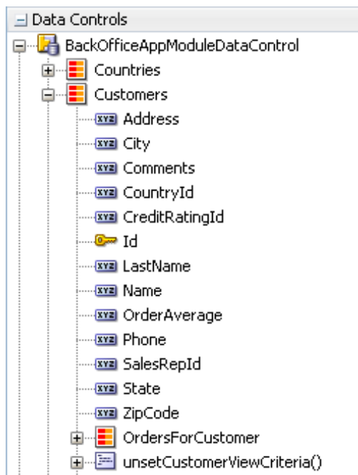
Figure 34-5 Master-Detail Objects in the Data Controls Panel
