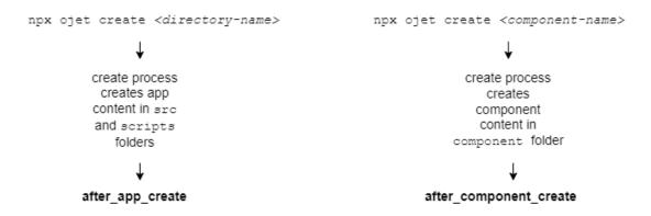
The following diagram shows the script hook point flow for the build process.
