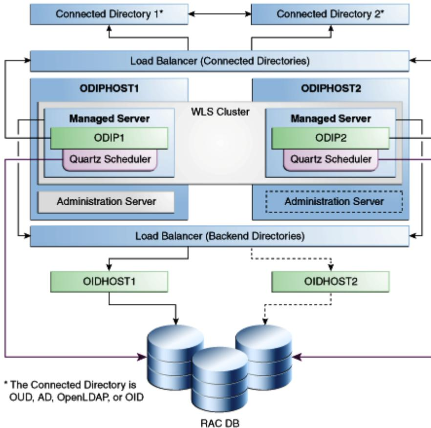
In [Figure 12-2](#), Connected Directory 1 and Connected Directory 2 replicate information with each other. A load balancing router routes requests to the Connected Directories.
