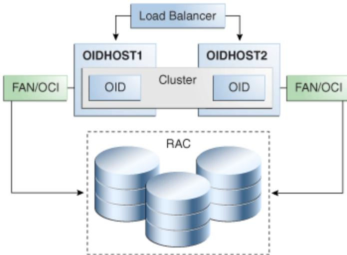
The [Figure 12-1](#) shows Oracle Internet Directory (OID) in the directory tier in a Cluster Configuration high availability architecture. Clustering is set up at installation time. The load balancing router routes LDAP client requests to the two OID instances that are clustered on `OIDHOST1` and `OIDHOST2`.
