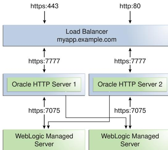
The load balancer receives user requests and forwards them to connected Oracle HTTP Servers. The load balancer receives requests on standard HTTP/HTTPS ports (80/443). However, it then passes requests to Oracle HTTP Servers using completely different ports. Advantages of this setup are:
