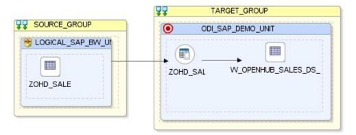
2. In the target group, select the access point for the source group that contains Open Hub Destination Table ZOHD\_SALE. This source group represents the source dataset made up of SAP BW Open Hub table.
