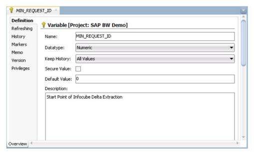
2. The value of this variable is updated at the end of the delta extraction package described in the third step. It happens once delta extraction is finished and the MAX REQUEST ID will be fetched from SAP BW system and will be stored into the ODI Variable (MIN\_REQUEST\_ID). The refresh expression shown here is used to update the variable:
