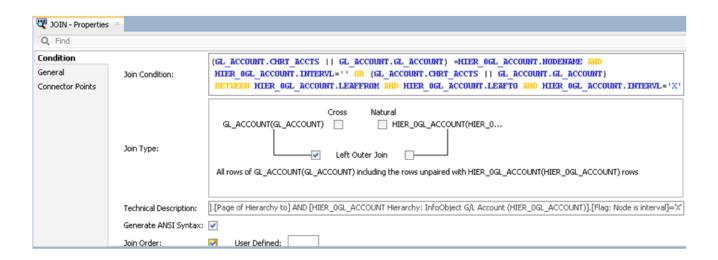
The final join and filter setup should look like this:
