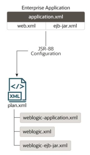
Figure 1-1 Configuring Applications with the Jakarta EE Deployment API
