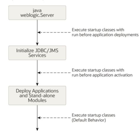
Figure 9-1 Startup Class Execution
