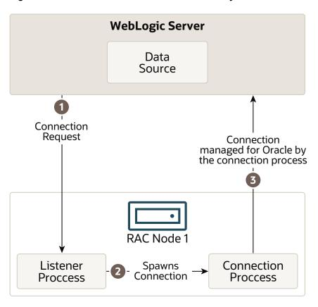
Figure B-3 Oracle Listener Process Functionality
