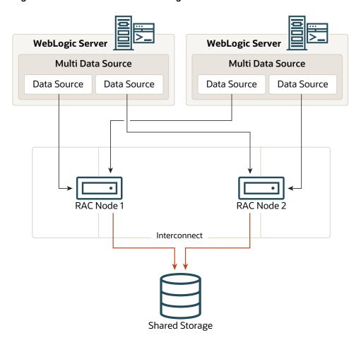
Figure B-2 Multi Data Source Configuration
