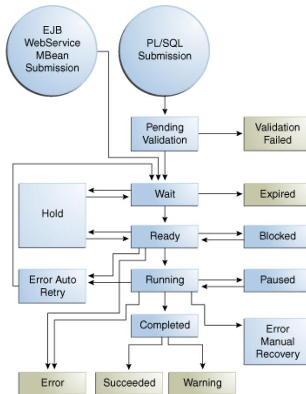
Figure A-3 displays the changes in state for an executable job request for which the executing user has canceled the request.
