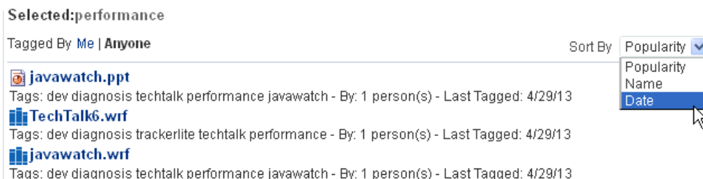
Figure 32-13 Tagged By and Sort By Options for Tagged Pages in the Tag Center
