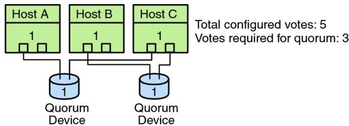
**In this configuration, usually applications are configured to run on Host A and Host B and use Host C as a hot spare.**
