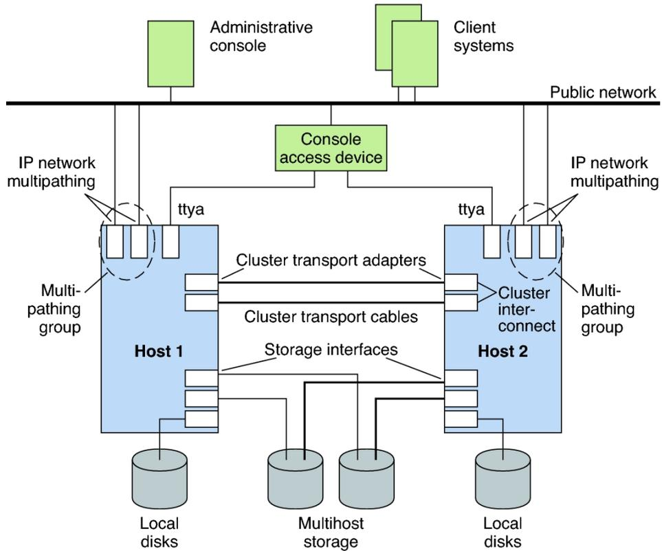
Administrative console and console access devices are used to reach the cluster nodes as needed. The Oracle Solaris Cluster software enables you to combine the hardware components into a variety of configurations. The following sections describe these configurations.
