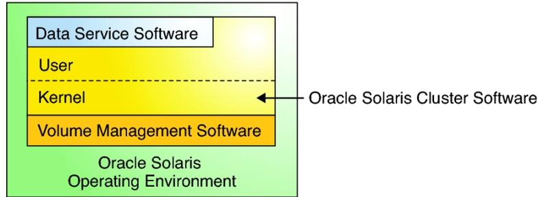
Figure 3, “Oracle Solaris Cluster Software Architecture,” on page 24 shows a high-level view of the software components that work together to create the Oracle Solaris Cluster software environment.
