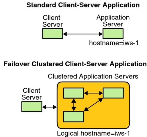
A shared address is also initially associated with one node. This node is called the global interface node. A shared address (known as the *global interface*) is used as the single network interface to the cluster.
