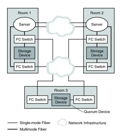
FIGURE 3 Basic Three-Room, Two-Node Campus Cluster Configuration With Multipathing
