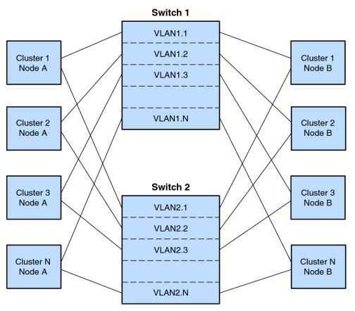
The second VLAN configuration uses the same transport junctions for the interconnect traffic of multiple clusters. However, the second VLAN configuration has two pairs of transport junctions that are connected by links. This configuration enables VLANs to be supported in a campus cluster configuration with the same restrictions as other campus cluster configurations. The following figure illustrates the second VLAN configuration.
