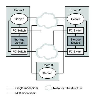
FIGURE 5 Three-Room, Three-Node Campus Cluster Configuration
