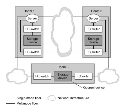
FIGURE 7 Three-Room Campus Cluster With a Multipathing Solution Implemented
