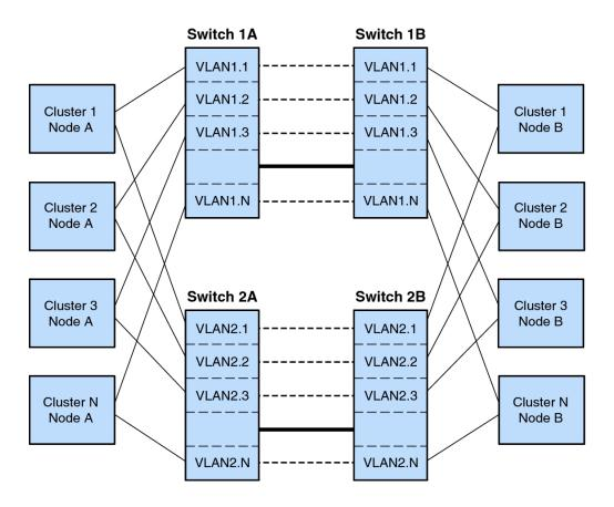
FIGURE 2 Second VLAN Configuration
