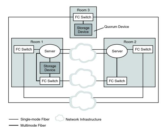
In Figure 5, "Three-Room, Three-Node Campus Cluster Configuration," on page 60, one room contains one node and shared storage. A second room contains a cluster node only. The third room contains shared storage only. A LUN or disk of the storage device in the third room is configured as a quorum device.
