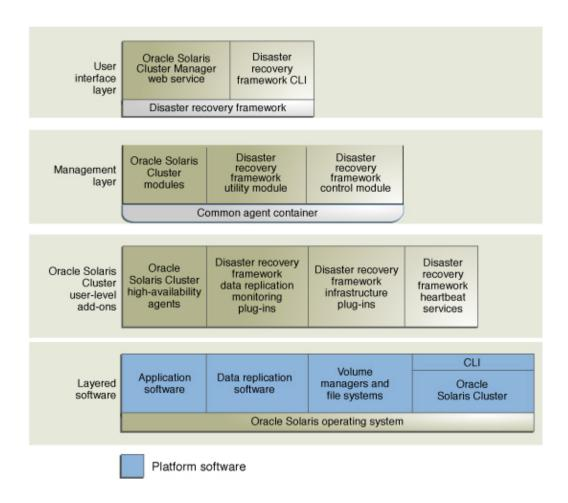
The clusters in a disaster recovery framework configuration can run different versions of Oracle Solaris Cluster software, as long as the versions are no more than one consecutive release different. For example, the clusters in one disaster recovery framework configuration could run either version 4.2 or 4.3, or run either version 4.2 or 4.1. But you cannot have clusters running either version 4.1 or 4.3 in the same disaster recovery framework configuration.
